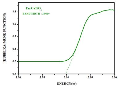
Fig .6. Optical band gap calculation of Eu :CaTiO<sub>3</sub> nanopowder prepared by sol-gel method
