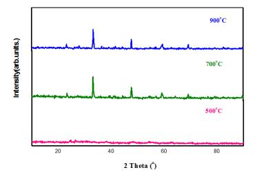
Fig.1. XRD pattern of Eu:CaTiO<sub>3</sub> nanopowder annealed at different temperature
