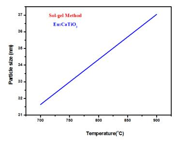
Fig.2.Particle sizes as a function of heat treatment of Eu:CaTiO<sub>3</sub> nanopowder synthesized by sol-gel method
