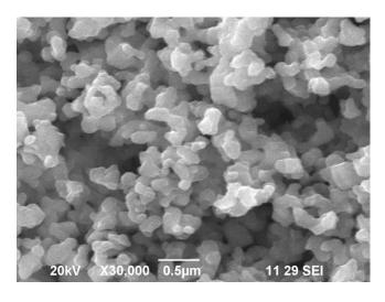
Fig.4 .SEM analysis of Eu :CaTiO<sub>3</sub> nanopowder prepared by sol-gel method
