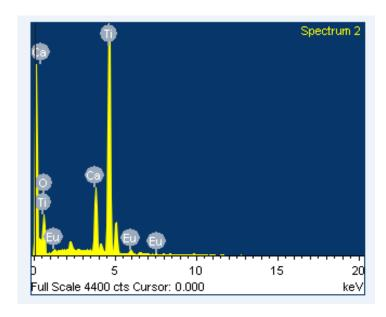
Fig. 5. EDAX analysis of Eu:CaTiO<sub>3</sub> nanopowder prepared by sol-gel method
