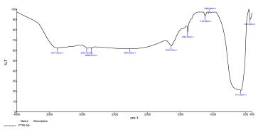
Fig.3 . FTIR spectra of Eu : CaTiO<sub>3</sub> nanopowder prepared by sol-gel method
