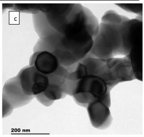
Fig. 7 a,b.c: HRTEM micrographs of Eu:CaTiO<sub>3</sub> nanopowder prepared by sol-gel method calcined at 900°C
